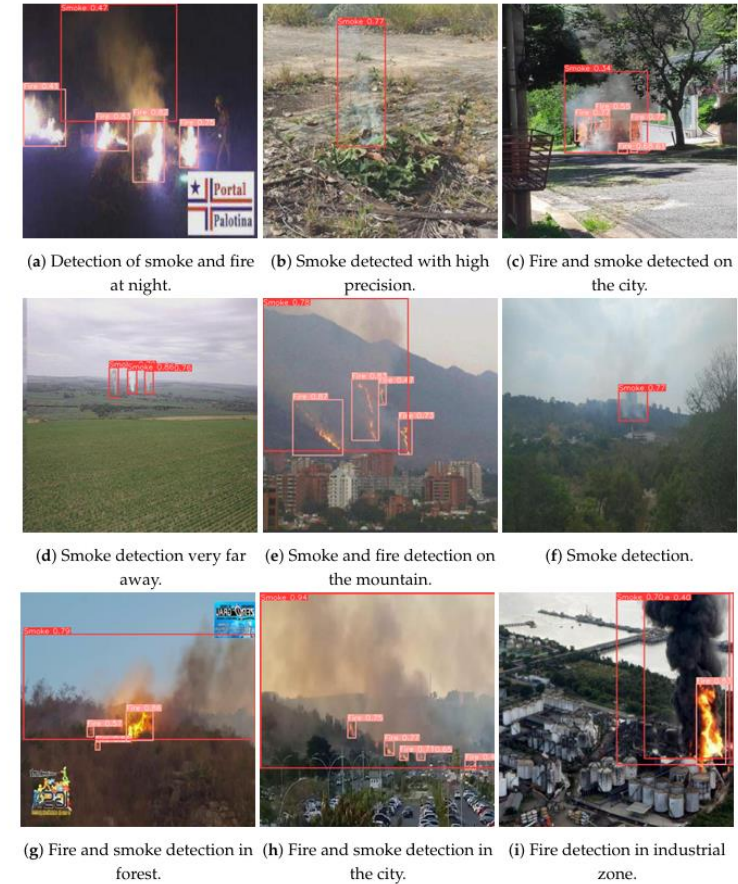
Figure 5. Example of fire and smoke detection by YOLOv8x model.
